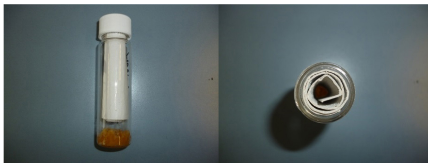
Figure A15: Food (marzipan) and recycled cardboard in the vial; side view, closed vial (left) and top view, open vial (right)
